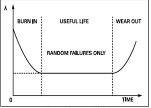
Figure1.0 Component life Failure
