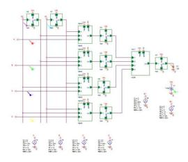
Fig.5 Schematic view of 4:1 Multiplexer with logical effort
