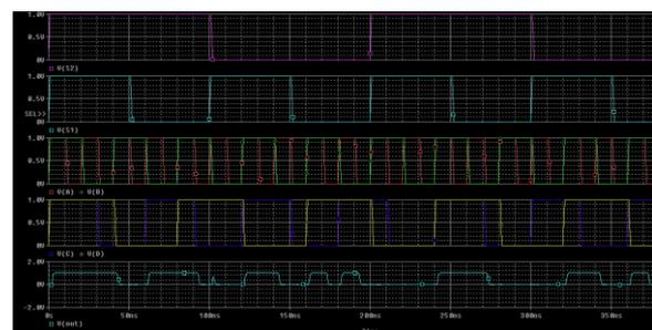
**Fig.4 Waveform of 4:1 multiplexer**
