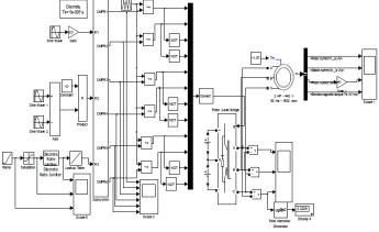
Fig19: Simulink block of Scalar Control
