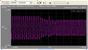
Fig. 14. Motor current when frequency transitioned from 40 to 50Hz(2 A/Div).
