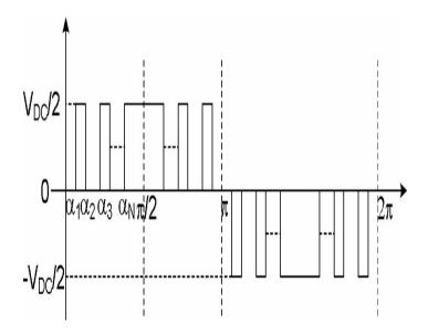
Fig. 3. Typical quarter-wave symmetric output voltage of a three-level NPC inverter leg.
