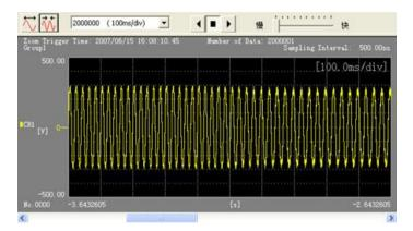
Fig. 17. Motor line voltage when frequency transitioned from 50 to 40Hz (100 V/Div).
