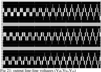
From this waveform, we observe that it is clearly seen that the wave form changes from two level voltage level to three level as frequency increases from 5 to 50 hertz
