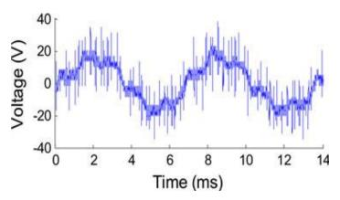
Fig. 8. Waveform of motor neutral point to dc-link midpoint voltage (20V/Div) at 50Hz with passive filter.
