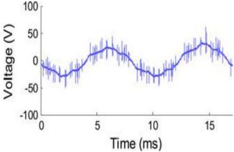
Fig. 12. Waveform of motor neutral point to dc-link midpoint voltage (50V/Div) at 40Hz with passive filter.
