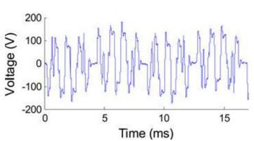
Fig. 10. Waveform of motor neutral point to dc-link midpoint voltage (100 V/Div) at 40 Hz without passive filter.
