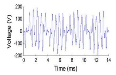
Fig. 6. Waveform of motor neutral point to dc-link midpoint voltage (100 V/Div) at 50 Hz without passive filter.
