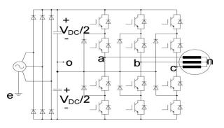
Fig. 1. Circuit diagram of three-level NPC induction motor drive with front- end diode rectifier.
