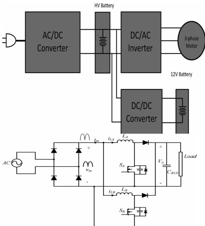
Fig. 2. Interleaved boost PFC schematic.
