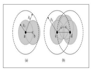
Figure.9: Communication Cases (a) Communication between a B-node and a G-node (b)Communication between two B-nodes.
