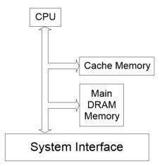
Fig.1: shows a simplified diagram of a system with cache. In this system, every time the CPU performs a read or write, the cache may intercept the bus transaction, allowing the cache to decrease the response time of the system. Before discussing this cache model, let's define some of the common terms used when talking about cache.
