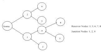
Fig. 1. A Multicast routing tree with 5 receivers and 3 intermediate junctions' nodes. ECN congestion is also not appropriate.
