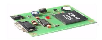
It operating at frequency range of 125 KHz. RFID reader with serial output with a range of 8-12cm. It is a compact unit with built in antenna and can be directly connected to the PC using RS232 protocol. A passive tag consists of three types: an antenna, a semiconductor chip connected to the antenna. The
