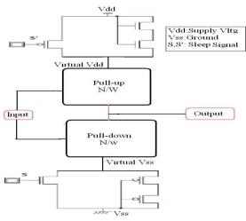
Fig6: Dual Stack Technique
