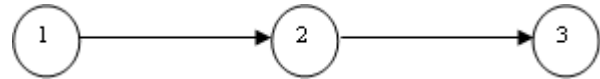
Fig.3. Two-link tandem network. Nodes 1 and 2 are each capable of injecting a single packet per unit time on their respective outgoing links.
