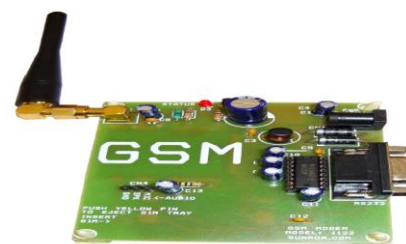
Figure. 4: Sunrom GSM modem
