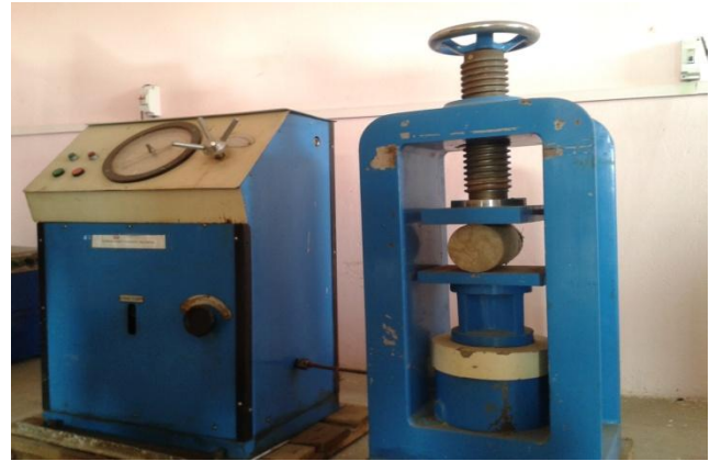
Figure 2(a): Split tensile test on concrete Cylinders
