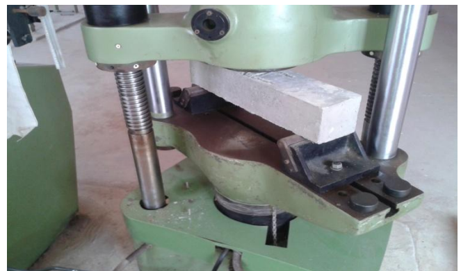
Figure 3(a): Flexure test of concrete prisms
