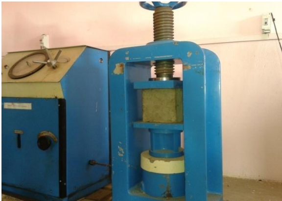
Figure 1(a): Compression test on concrete cubes
