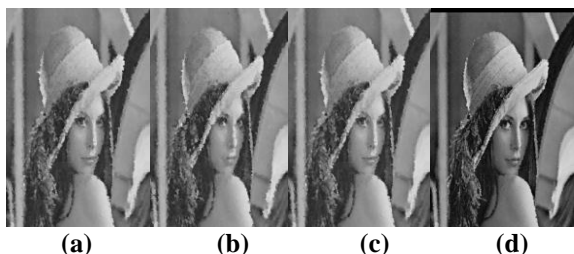
Figure 2: Results of different filters when the image is corrupted with 90% of salt and pepper noise. a) Output of DBUTMF, b) Output of IAEF, c) Output of ISF d) Output of MNASMF.
