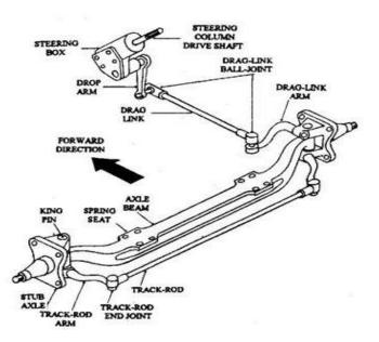
Figure 2: Front axle beam linkage assembly with Steering system
