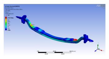
Figure 5: Analysis of equivalent (Von-mises) stress
