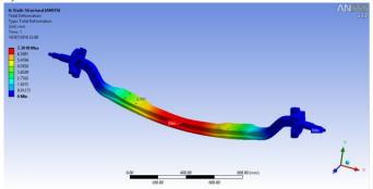
Figure 6: Analysis of total deformation
