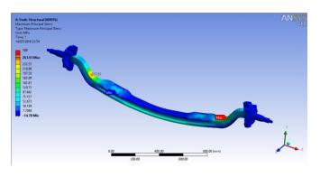
Figure 4: Analysis of Maximum Principle Stress
