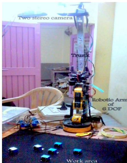
Figure 1: A Pick and Place robot. A six DOF manipulator arm is mounted on a trunk which is fixed on a table. The robot possesses a stereo camera head.
