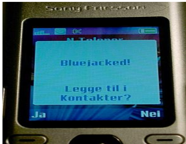
Fig. 2 what does receiver sees on the screen as it receives the bluejack message [5]
