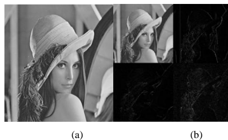
Figure 4 . (a) Original image-Lena (b) Result after the first-order 2-D Haar-DWT
