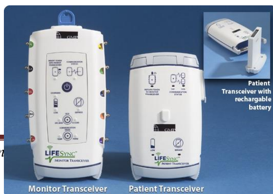
Fig.2 The patient transceiver (sensor unit) and monitor transceiver (receiver unit) of the LifeSync Wireless ECG System [11].
