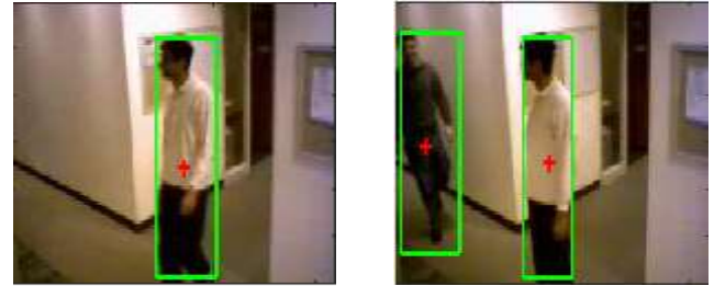
Figure 9: Tracking results for centroid based object tracking frame # 85 and frame # 131
