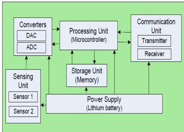
Fig 1.1- The Components of a sensor node.
