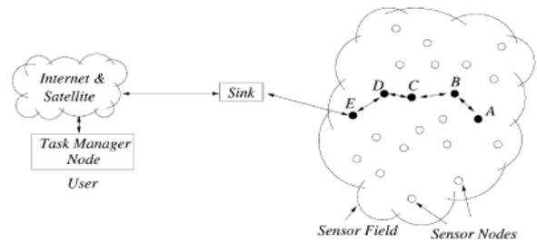
Fig 1.2-Wireless Sensor Network Architecture
