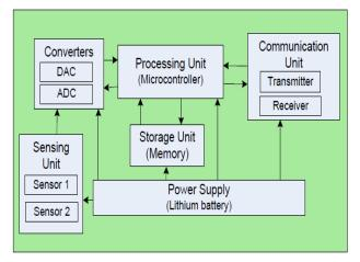
Fig 1.1- The Components of a sensor node.
