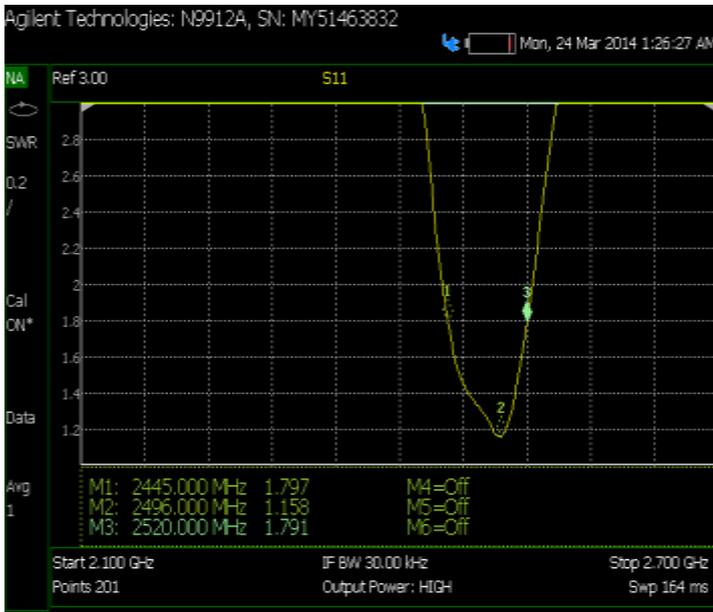
Figure 10 Measured VSWR result of PMC
