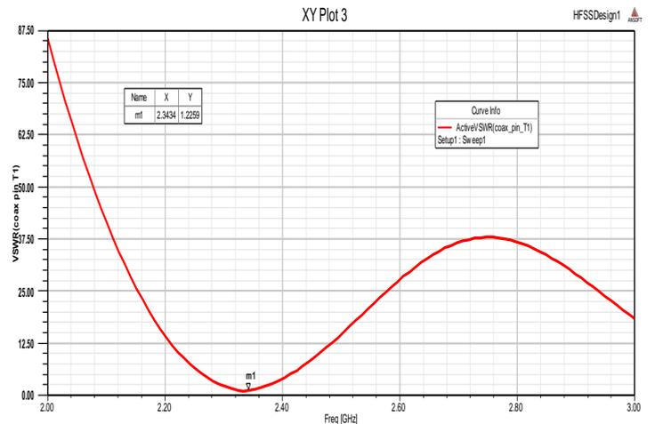
Figure 9 Measured VSWR result of PMC
