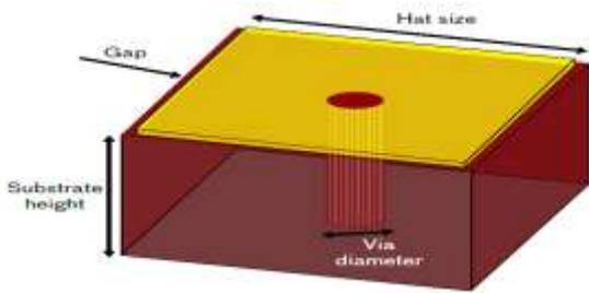
Figure 1 Constructional view of AMC Cell
