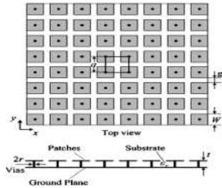
Figure 2 Top view of AMC
