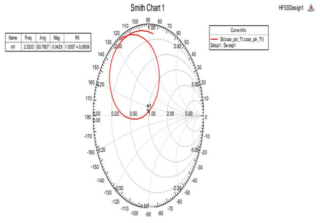
Figure 7 Simulated result of impedance using smith
