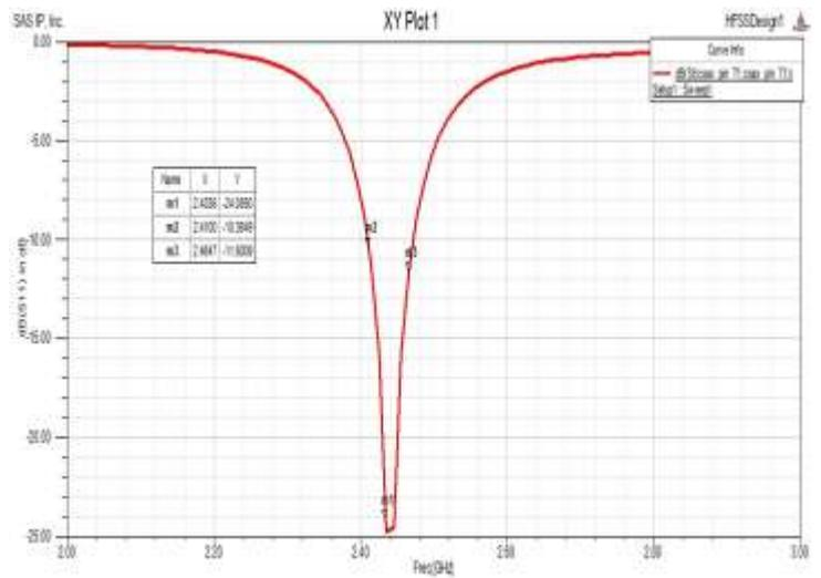
Figure 4 Simulated Return Loss (S11) of PMC
