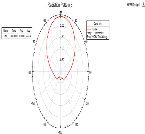
Figure 6 Shows directivity of PMC antenna.
