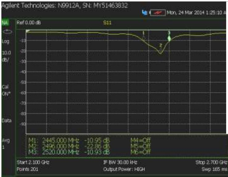
Figure 5 Measured Return Loss (S11) of PMC
