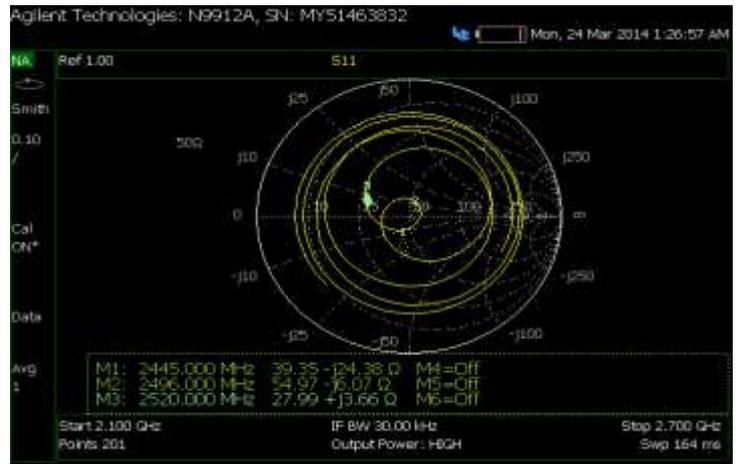
Figure 8 Measured result of Smith chart on VNA
